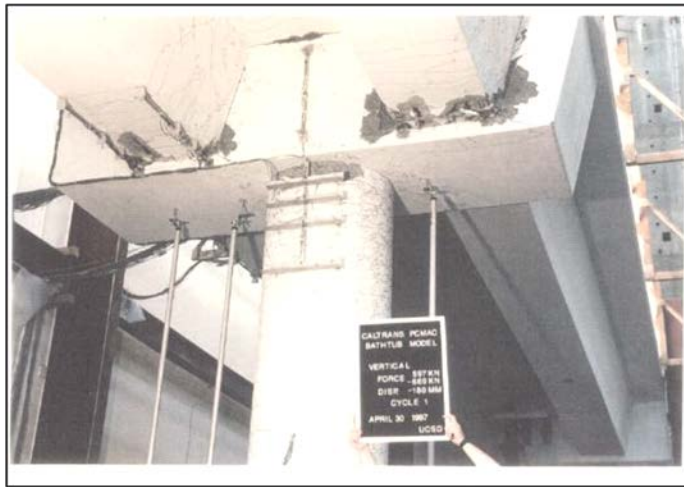
Figure 2.12: Bathtub test unit (Holombo, 1999)
