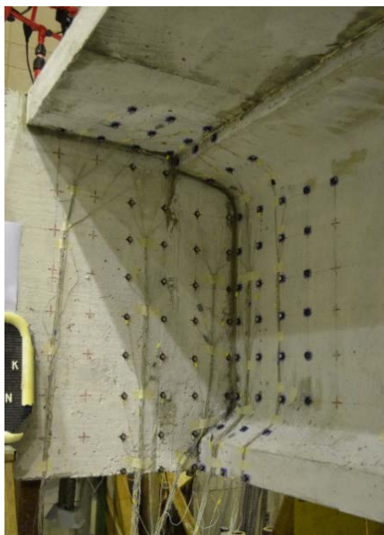
Figure 3.34: LED configuration at connection region
