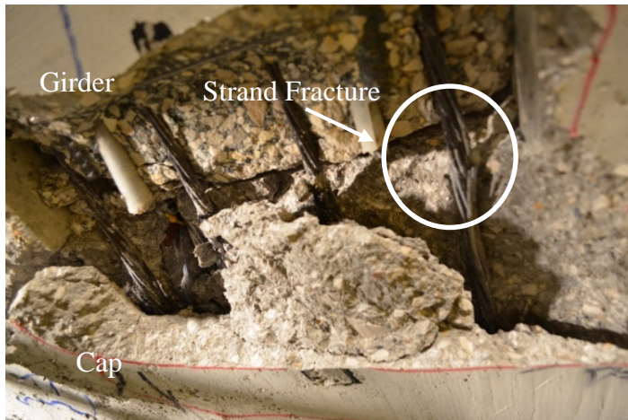
Figure 4.8: Partial extended strand fracture
